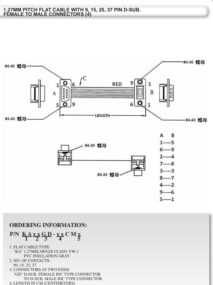
5. NUT OPTION AT TWO CONNECTORS: "N" WITH UNC4-40 NUTS "W" WITHOUT NUTS
